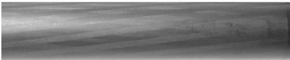
***Spun carbon fibre.*** *The clarity of the 'grain' is no indicator of quality. Above is Redged (very good); below, Gitzo (even better).*
