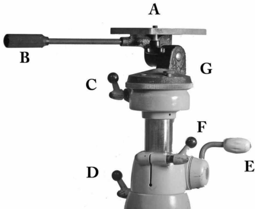
**Seven controls:** A, camera screw, B, pan lever and tilt lock, C, lock for removing head, D, lock for removing centre column (head can be placed directly on tripod), E, crank for centre column, F, lock for centre column, G (barely visible small screw on top of head base) pan lock.
