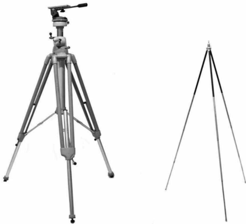
**Two tripods.** *The Linhof is the biggest, heaviest tripod we own, seen here at little more than half its maximum height. The Johnsons 'wobble-pod' is the smallest and lightest, except for table-tops. It is reproduced at the same scale as the Linhof, and is at full extension. But both have their place.*
