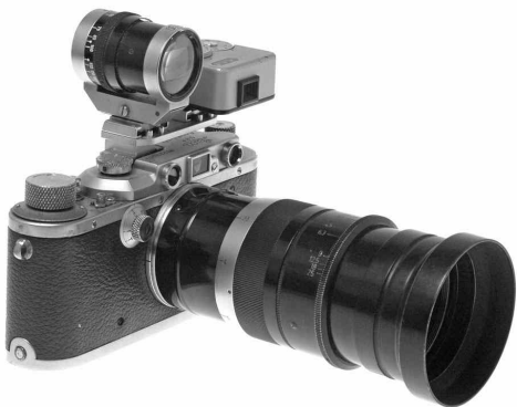
Accessory shoe doubler on 1936 Leica IIIa with 1938 90/2.2 Thambar, 1950s Tewe finder and 1990s Voigtländer exposure meter.
